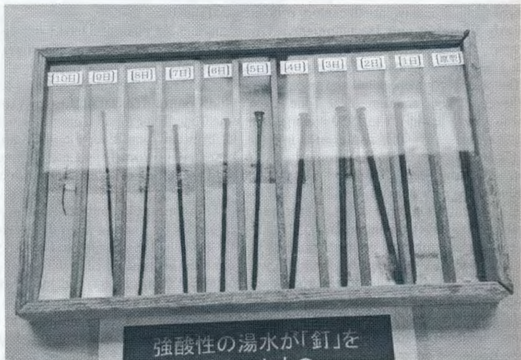
Fig. 3 Degeneration of nails in acidic Agatsuma River water (author's photograph)
